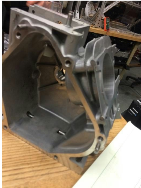
Figure 2: Briggs and Stratton “Animal” Engine, with engine head milled
