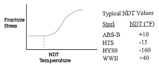
Figure 6 Illustration of Typical Fracture Behavior for Steels
