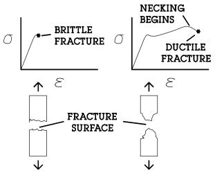
Figure 1: Brittle vs Ductile Fracture
