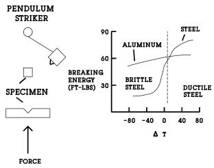
Figure 3: Charpy Impact Test
