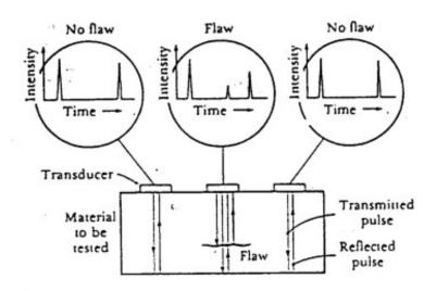
Figure 18 Ultrasonic Testing
