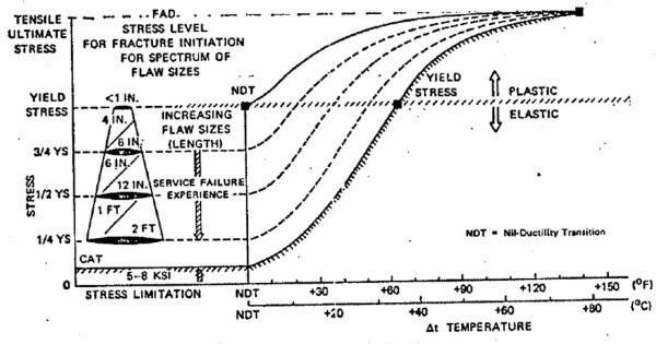
Figure 7: Fracture Analysis Diagram
