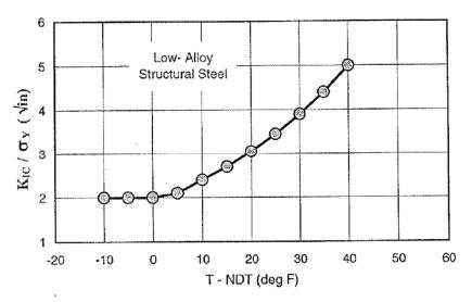
Figure 12. Variation in Fracture Toughness with Temperature
