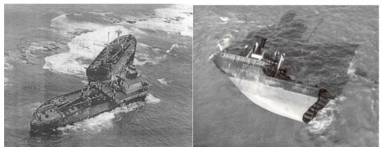
Figure 4. Fractured Hull of Liberty Ship
