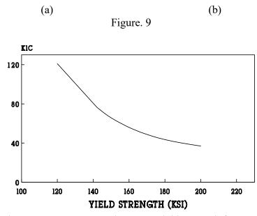
Figure 10: Fracture Toughness vs Yield Strength for Steel
