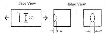
Surface Flaw Interior Flaw Fig. 11 Flaw Geometry
