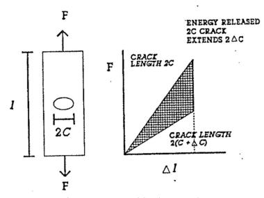
Fig. 8 Fracture with Thru Crack
