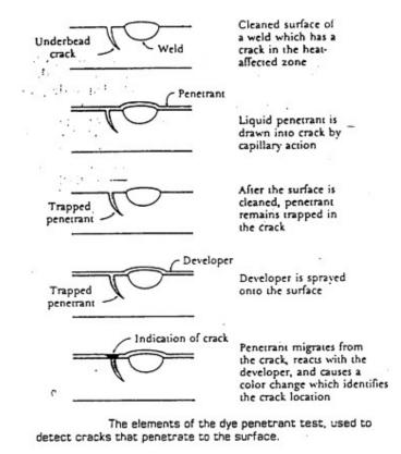
Fig 16: Dye Penetrant Testing
