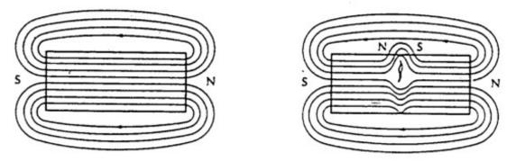
Figure 17 Magnetic Particle Testing
