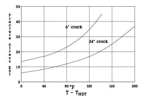
Figure 13: Fracture Toughness with Temperature
