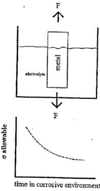
Figure 14: Stress Corrosion Cracking
