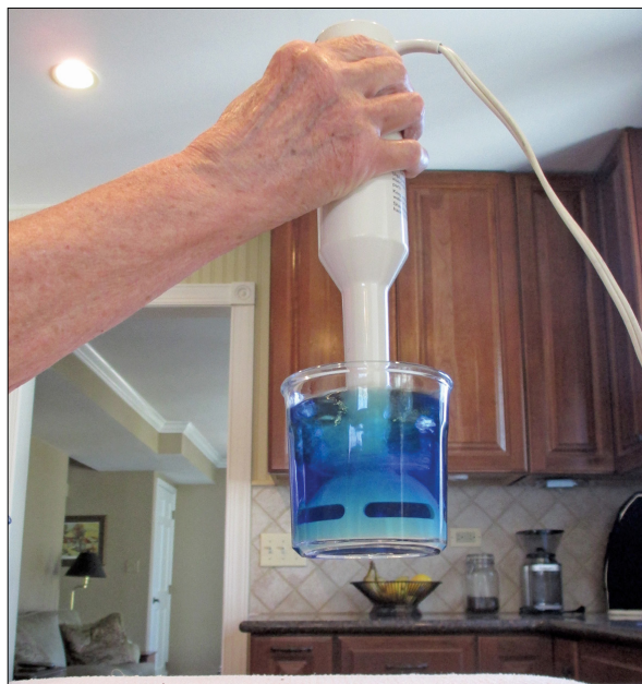
A glass of water being lifted with an immersion hand blender. The food coloring added to enhance the photo played no role in levitation.
