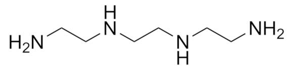
Structure of TETA, a typical hardener. The amine (NH) groups react with the epoxide groups of the resin during polymerization
