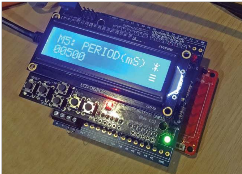
FIGURE 4 The full assembly of three boards, with the display on top showing one of the modes.
