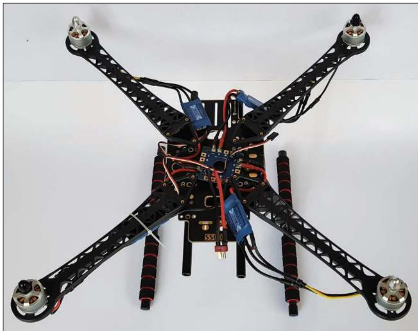
FIGURE 2 S500 frame with motors, ESCs and power distribution board
