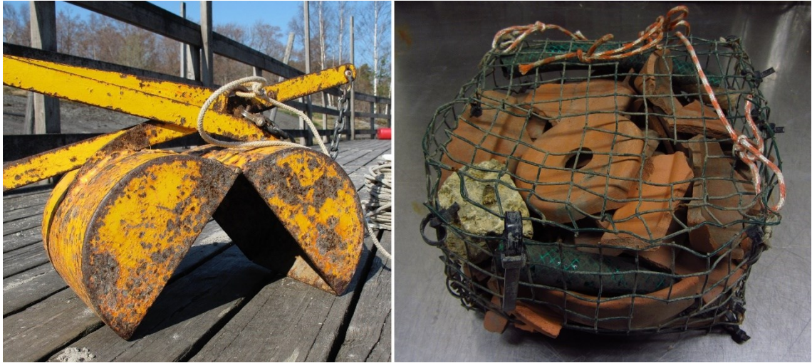
Figure 2. Mini Petersen grab and a type of non-catching habitat trap used in the sampling.
