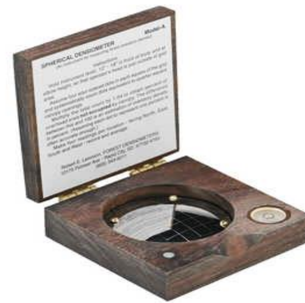
Figure 7 Convex glass densiometer for measuring tree canopy cover or shade.
