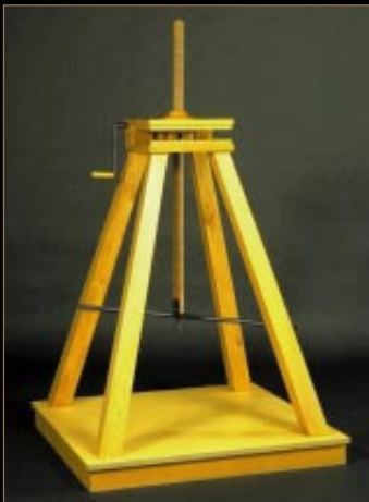
Leonardo da Vinci SCREW JACK WITH ANTIFRICTION BEARING
