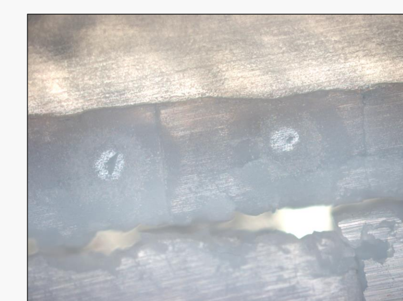
Optical microscope image of LIBS ablation craters on sectioned otolith.
