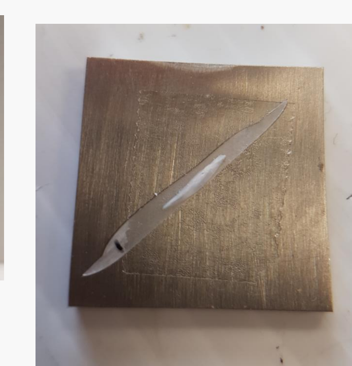
Otolith is cut through the marked origin with two diamond blades separated 0.39mm at 45°
