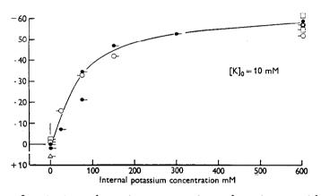
7. Effect of varying internal potassium concentration on the resting potential. External solution, sea water containing 10 mM K; internal solution NaCl-KC1 solutions isotonic with sea water. Note that the resting potential reaches a limiting value of about - 55 mV at potassium concentration greater than 150 mM. From Baker *et al.* 54.
