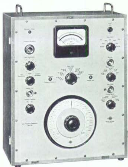
Fig. 10 Photo of a modern sound spectrum analyzer (Brüel & Kjær Audio Frequency Spectrometer Type 2112).
