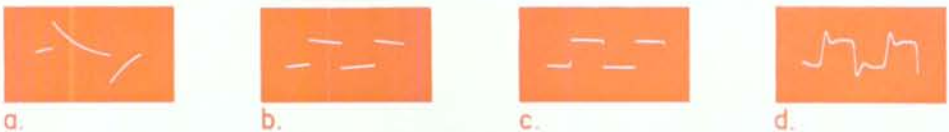
Fig. 8 Typical wave form distortion of a symmetrical square-wave treated in the amplifier (Frequency response 2 c/s—40 kc/s).
