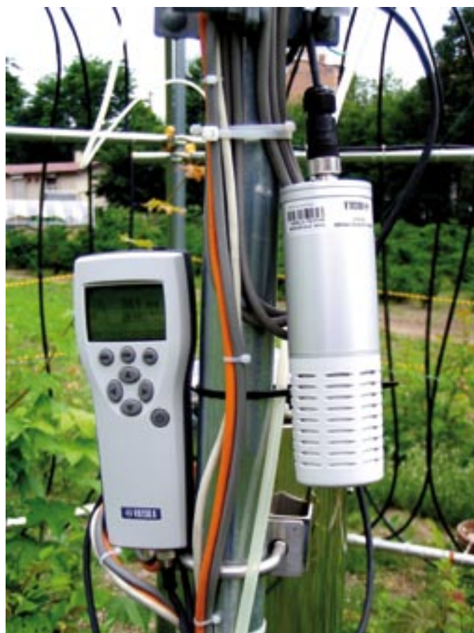
Figure 2: The Vaisala CARBOCAP® Carbon Dioxide Probe GMP343 inside the FACE.
