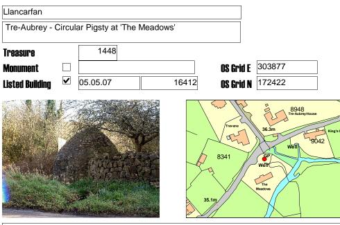
Traditional C18 corbelled pigsty constructed of coursed liassic limestone rubble with traces of limewash together with the remains of the pig pen with enclosing walls, also of limestone. The stone stile survives in the wall to the North of the sty.
