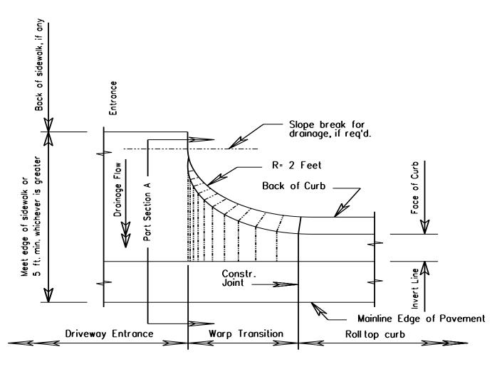
Part Plan of Entrance Transition FIGURE 7 - ROLL TOP CURB ENTRANCE DETAIL
