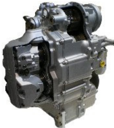
Figure 2: ZF CVT with double yoke hydro
