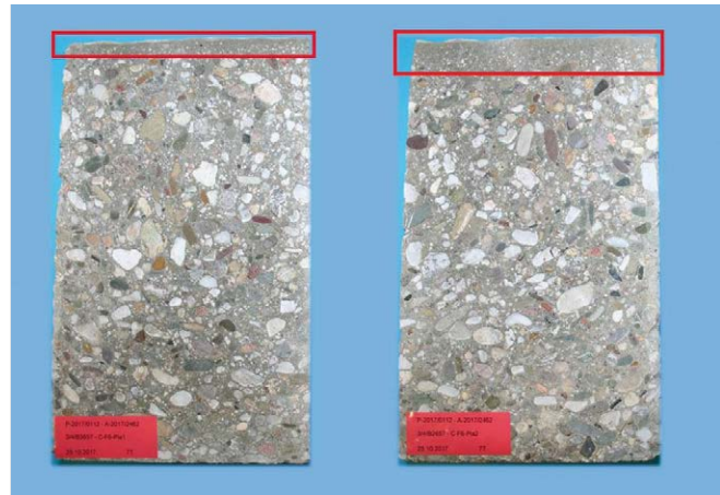
Fig. 3.4.15-2 Structure of concrete with high workability and low viscosity after compaction through squeegeeing (left) and after compaction on a vibrating table ( f = 50 Hz) in three layers, each layer vibrated for 20 s (right); framed areas: visible segregation of coarse aggregates
