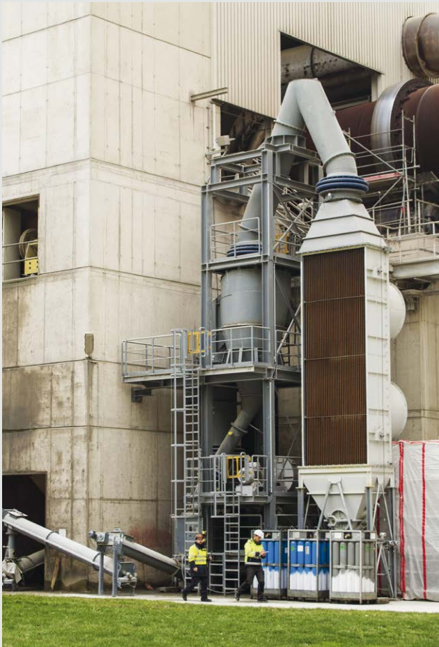
Fig. 1.3.1-1 Prototype oxyfuel clinker cooler undergoing practical testing
