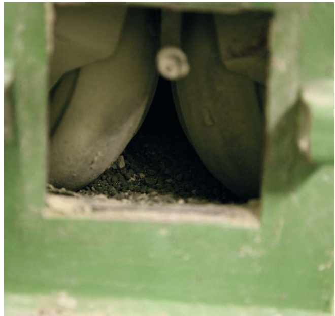
Fig. 3.1.1-2 Mill chamber of the small-scale vertical roller mill
