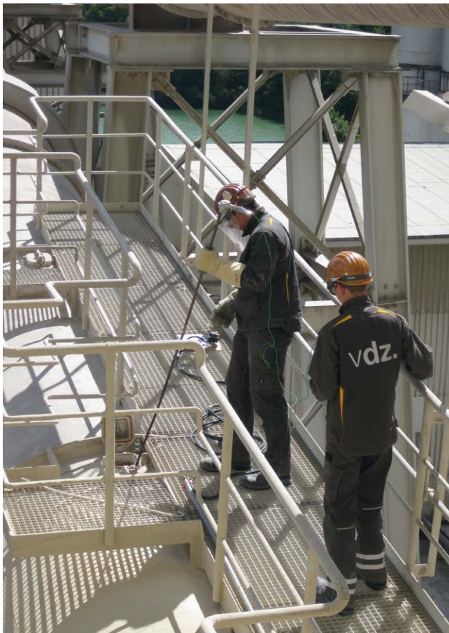
Fig. 3.1.3-2 Operational measurement of hot gas temperature
