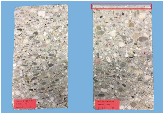
Fig. 3.4.15-1 Structure of concrete with high workability and mid-level viscosity after compaction through squeegeeing (left) and after compaction on a vibrating table ( f = 50 Hz) in three layers, each layer vibrated for 20 s (right); framed area: visible segregation of coarse aggregates
