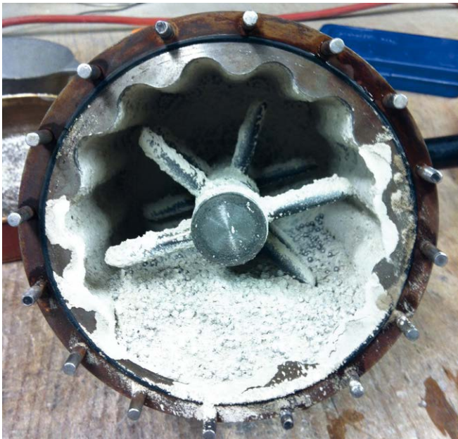
Fig. 3.1.1-1 Stirred media mill for separate superfine grinding
