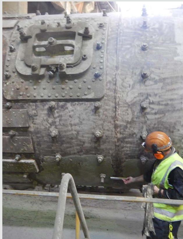
Fig. 2.1-3 Working on the ball mill built in 1959
