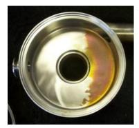
Besides the rouging by ultra-pure water, rouging can be formed by external compounds in a water environment. One common source is ferrous bicarbonate. This is commonly used to soften hard water (lower calcium concentration). By means of several chemical reactions and with or without chlorine disinfection, iron hydroxides and ferric oxides are formed and deposit as rouge. Dissolved carbon dioxide gas also contributes the formation of rouge in ultra-pure water systems..
