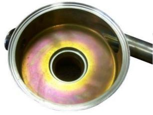
Pump casing with rouging before treatment
