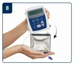
Connect the cassette by fitting the hooks onto the pivot pins at the base of the pump. Push the cassette up against the pump. Place the joined pump and cassette in an upright position on a steady surface. Secure the cassette by using a coin to turn the lock knob 90° counterclockwise until you feel it stop. Patients can now move to the section "A stepby-step programming guide"
