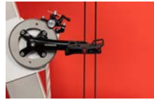
Knielot mechanisch fernsteuerbar Remote mechanical adjustment of the knee position.
