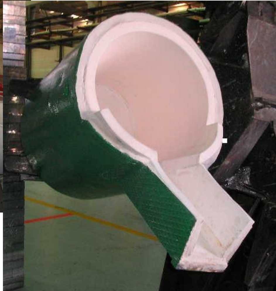
Refractory ladle: After Insural ATL 600
