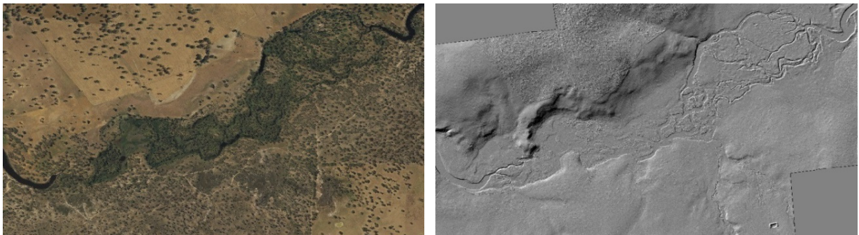
Photo 6: (a) and (b) Section of reach 1b upstream of Fulham Bridge (flow right to left), note the transition between a well-defined channel to multiple channels then a floodout feature with no defined channel before forming a single thread channel again (Alluvium, 2012). (Photos: Alluvium)
