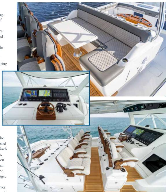
Port and starboard glove boxes house a variety of instruments and controls, including the fuel tank selector switches, Hooker live well variable speed control knobs and bow thruster control. Above, you have a molded-in pod in the hardtop for VHF radios and monitors and controls for various systems, such as the Seakeeper, water maker and a Garmin marine instrument display.
