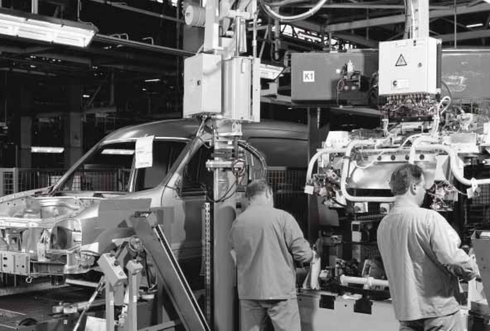
Automation of hardware fitting lines at the Renault plant in Maubeuge which produces the Kangoo.
