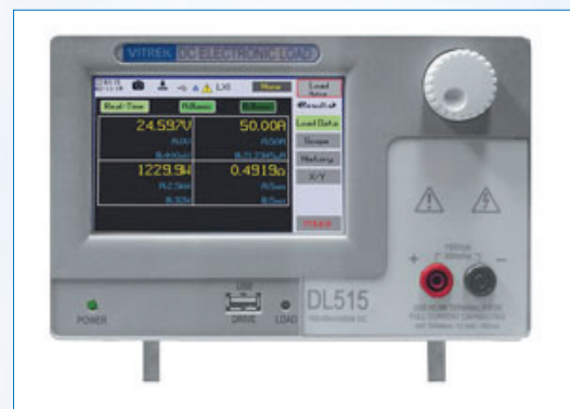
Figure 11. Vitrek DL Series Electronic DC Load
