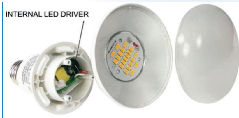
Figure 1. If a driver is integrated into an LED fixture, the input and output power must be monitored to measure against the IES LM-79-19 specification for driver efficiency.
