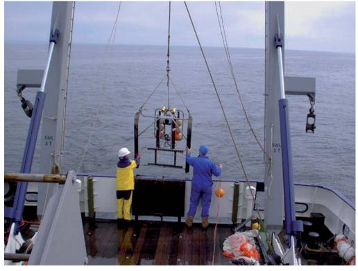
B. Deploying the camera sledge. Note the yellow USBL range locating acoustic transducers attached to the sledge on the May 2005 cruise.
