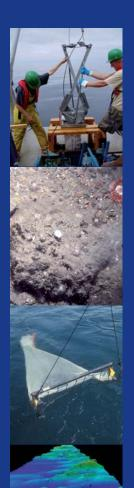
Van Veen grabs were deployed to obtain samples from the sea bed for investigation of fauna and sediment type.
