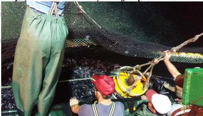
Figure 3. Opening the slipping net and pumping of the fish in the bunt by a fish pump.
