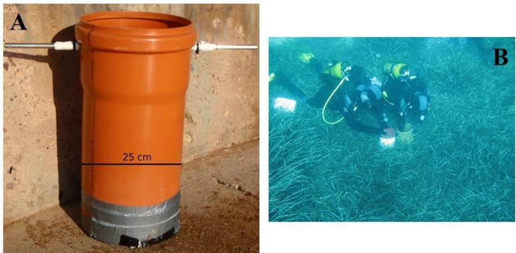
Figure 2.8: Standardized sampling. A: 25 cm diameter PVC “litter core” used for standardized sampling. B: A team of two divers applying the protocol, one holding the sealed plastic tanks, the other using the PVC cylinder for manual sampling.
