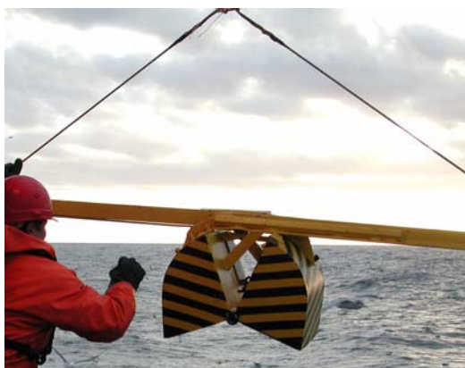
Fig. 4.2: Photograph showing the grab used for sediment sampling during the cruise WH268.
