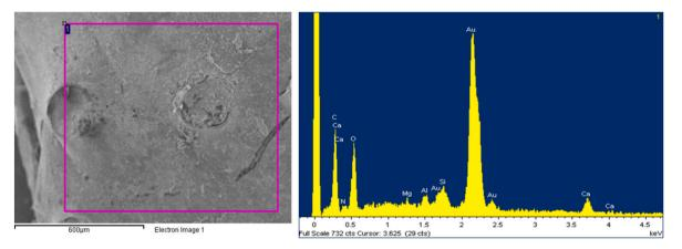
Fig. 7. Microanalysis of Watersipora subatra. The X-ray spectrum of dispersive energy represents the counts of x-ray photons emitted by each element of the sample.
