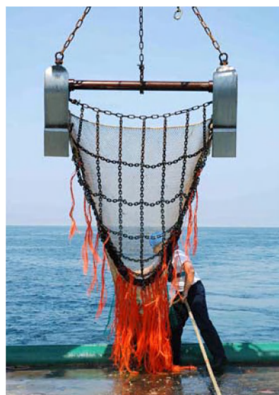
Figure 3-3. 2m beam trawl on rear deck of the R/V Belgica, spring 2005. Photograph : M. Fettweis, MUMM.
