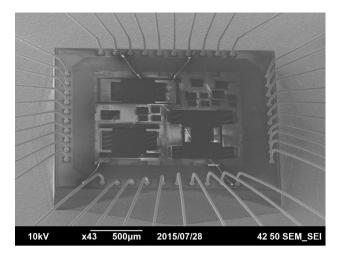
Fig. 11 Packaged chip after MEMS post-processing
