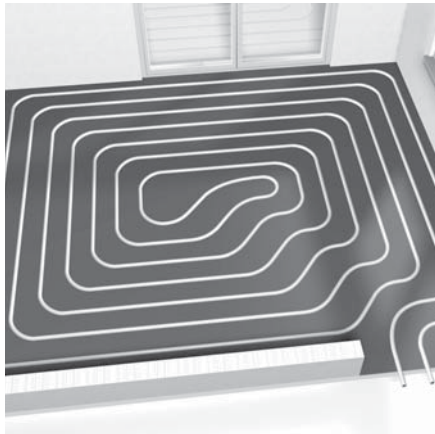
Figure 2: Snail's shell installation pattern
