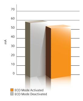
4. For many years, Gigaset DECT handsets have enabled the automatic adjustment of transmission power - depending on the distance to the base station. For example, transmission power is reduced by approximately 60% at a distance of up to five metres.
