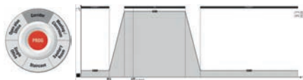
Possible DALI solution for applications in corridors: DALIeco with activated corridor function (2 changing lighting values)
