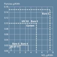
Within the EU, emission requirements for heavy diesel vehicles are regulated through the so-called Euro classes. Vehicles registered after October 1, 2006 will have to fulfill the Euro 4 emissions standard, while the Euro 5 standard will come into effect on October 1, 2009. The EU standards are designed to harmonize with standards that will come into effect in the US. Volvo welcomes a more rapid harmonization of European standards with American ones.
