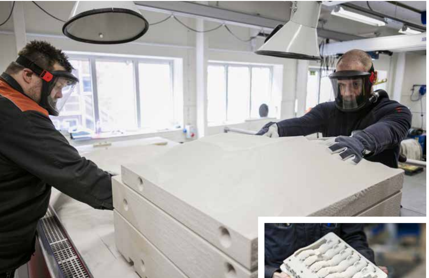
Operators Johan Arvidsson (left) and Lars Widhensparr are working on removing the sand from the finished cores. The process of producing 3D sand cores is faster than working with traditional methods because the process involves fewer stages.
