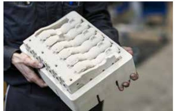
Operators Johan Arvidsson (left) and Lars Widhensparr are working on removing the sand from the finished cores. The process of producing 3D sand cores is faster than working with traditional methods because the process involves fewer stages.
