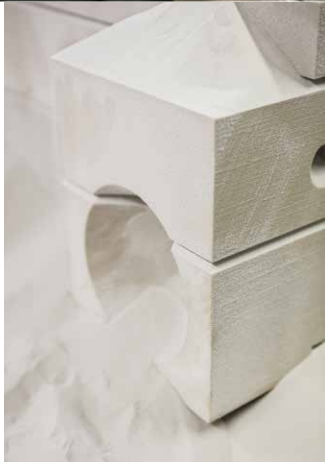
These finished cores are about to be sanded off by the operators. The cores are then used to cast metal component prototypes. Each layer of sand in the core is 0.3 mm thick and is interspersed with a thin layer of glue.
