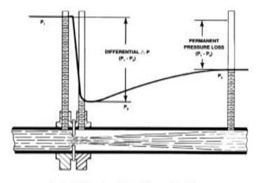
Typical Orifice Flow Pattern Flange Taps Shown
