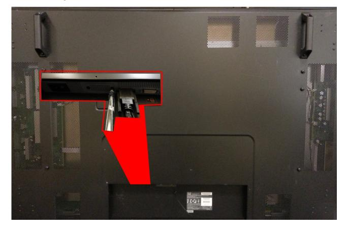
**c.** Press the button underneath the cover to enter factory mode.
