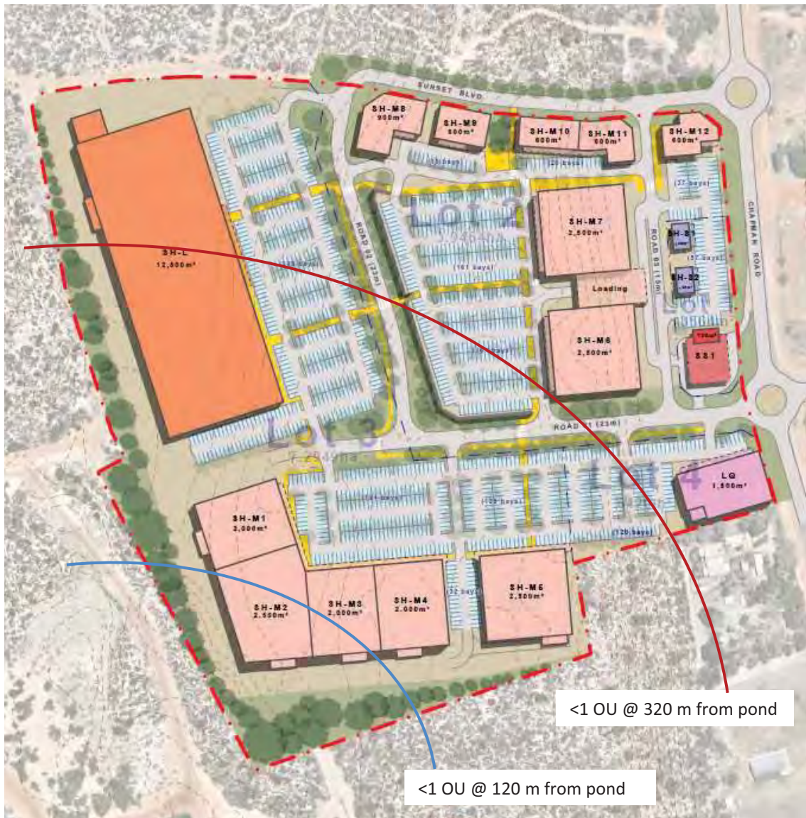
Figure 9: Site concept drawing showing illustration of odour impact with distance from the WWTP
