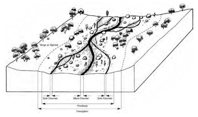
Figure 4. Cross section of a typical river valley and the terms used to describe it (Source: Pen and Scott, 1995)
