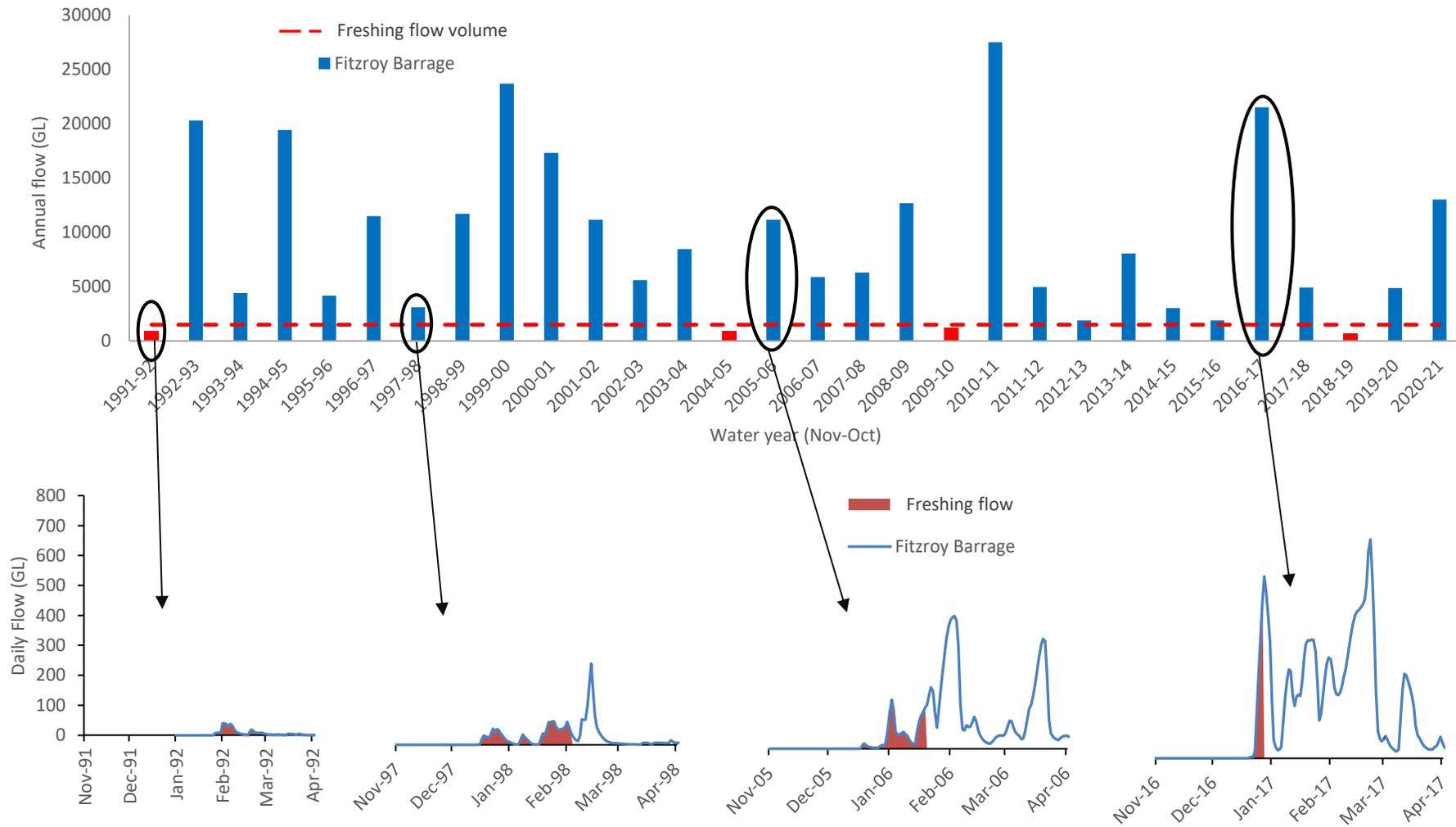
Figure 15 Annual flow at the Barrage from 1991–2021, highlighting freshening flows under 1,500 GL and how this would look in years with varying total flows
