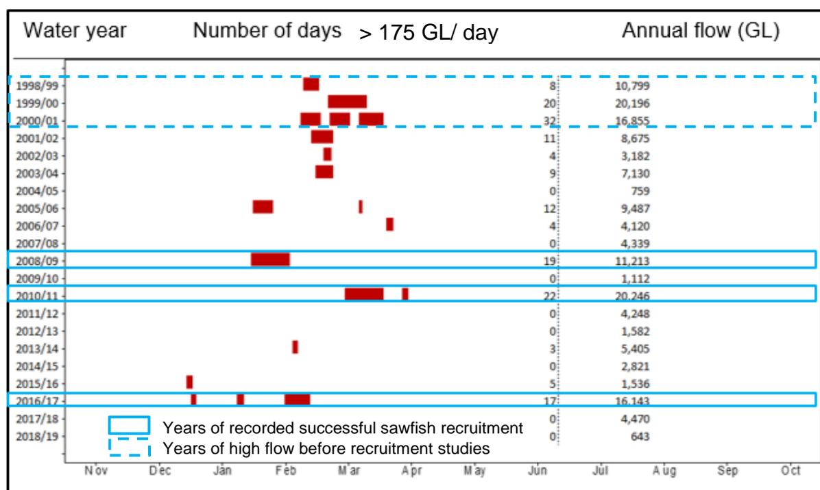
Figure 19 Duration of ‘high-flow’ conditions suitable for sawfish in days each year from 1998–1999 to 2018–2019 measured at Willare gauging station (802008)
