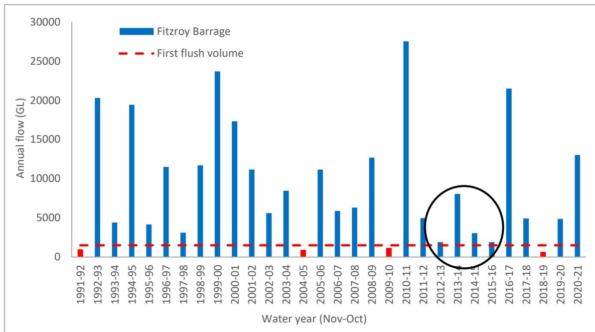
Figure 22 Years (1991–2021) when very low flow occurred (<1500 GL) and series of low-flow (dry) years from 2012–2013 to 2015–2016
