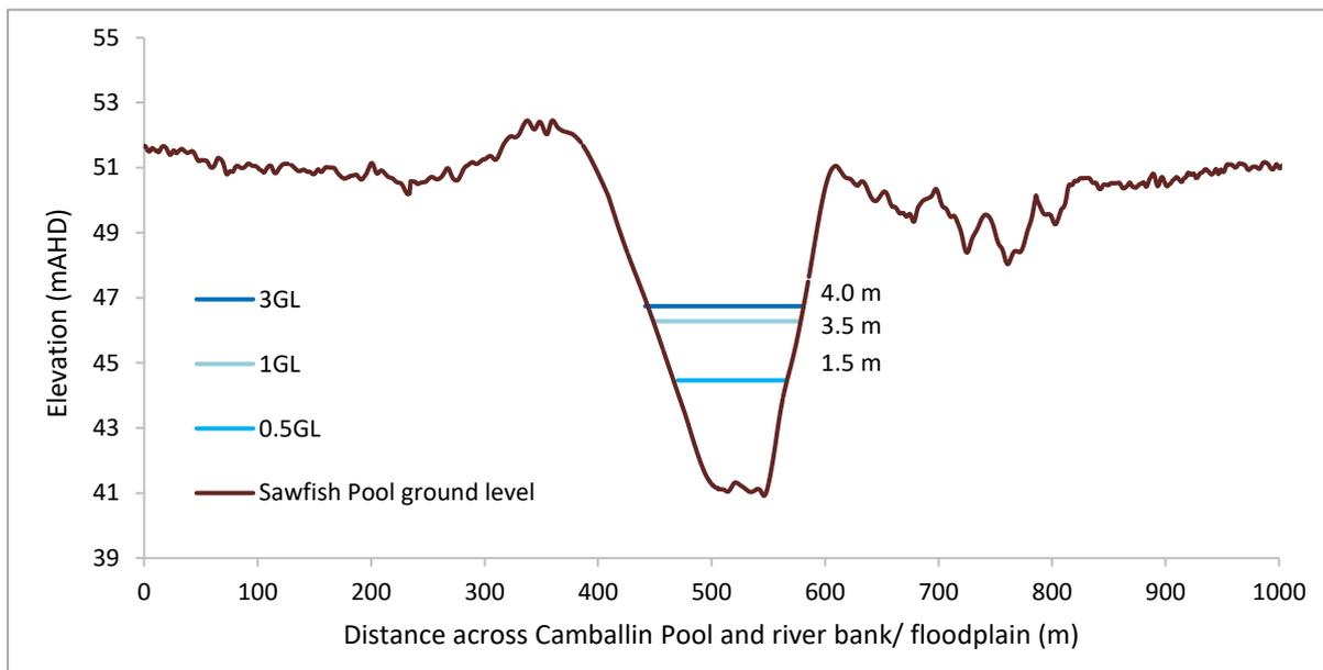
Figure 17 Modelled depth of Camballin Pool under different flow rates
