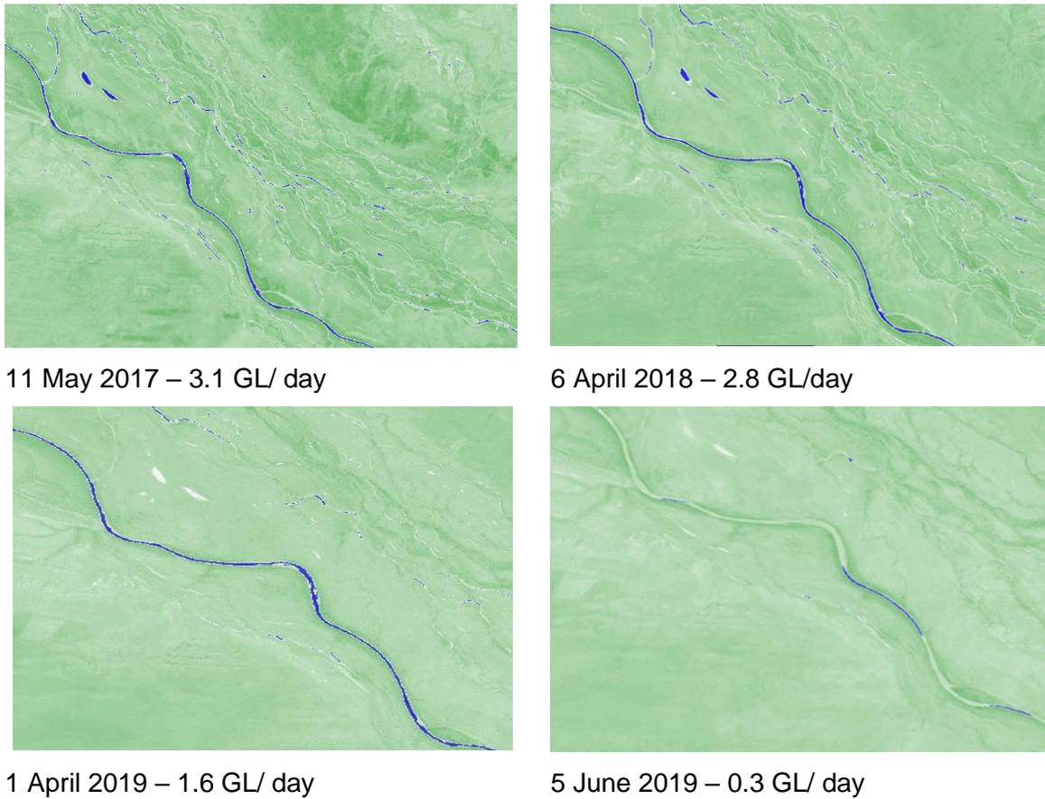
Figure 16 Presence of water downstream of Looma gauging station at various flow rates measured at the Fitzroy Barrage gauging station
