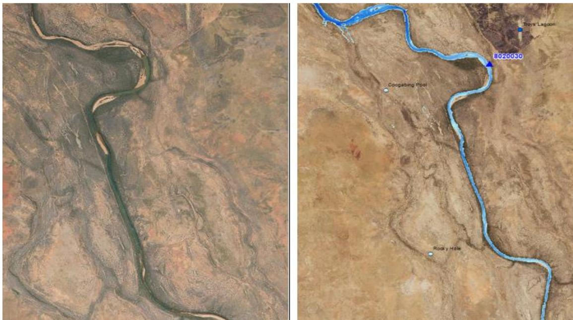
*Figure 14 Pool connectivity upstream and downstream of the Fitzroy (Camballin) Barrage at no flow (left) and 1,500 GL (cumulative)(right)*
