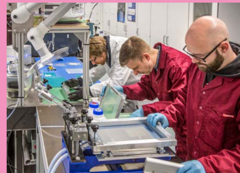
Production of plasma devices for accelerating wound healing at Coldplasmatech. The large silicone dressing can be seen in the center.
