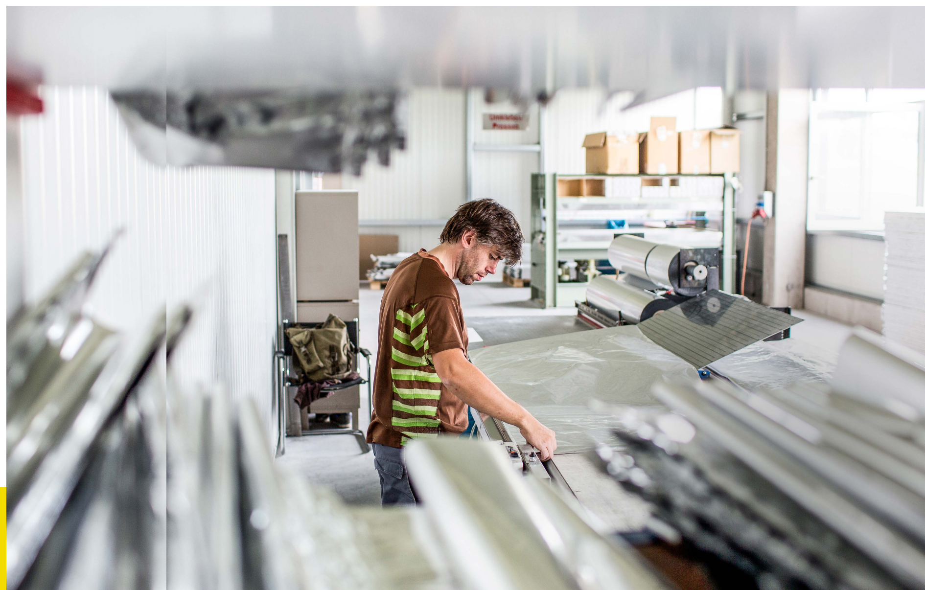
An employee fits the the molded panel made from the HDK® blend into a specially designed foil bag and then applies a vacuum to it.
