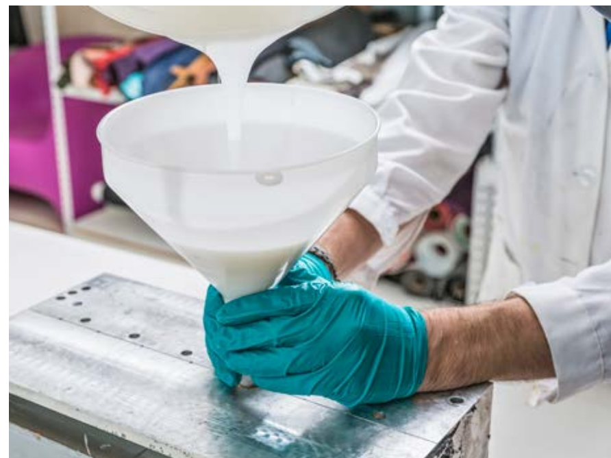
Simplicity Works employees demonstrating how the silicone material provided by WACKER is poured to create the patented 3D bonding silicone mold.
