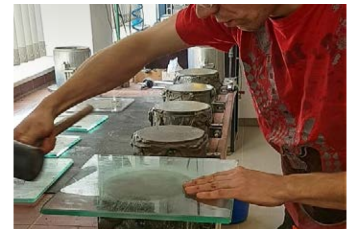
Test specimens being prepared for the analysis of mechanical strength at STRABAG's test center.
