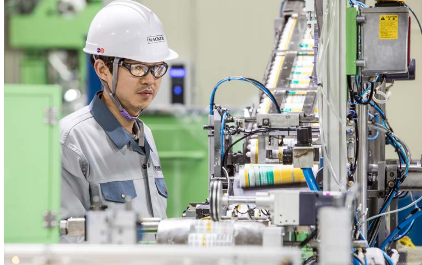
Filling up cartridges with silicone sealant at WACKER's new site in Jincheon, South Korea.
