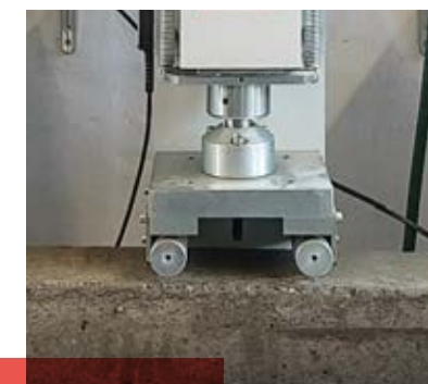
The flexural strength of a soil sample being tested at STRABAG's "TPA" quality-assurance laboratory.
