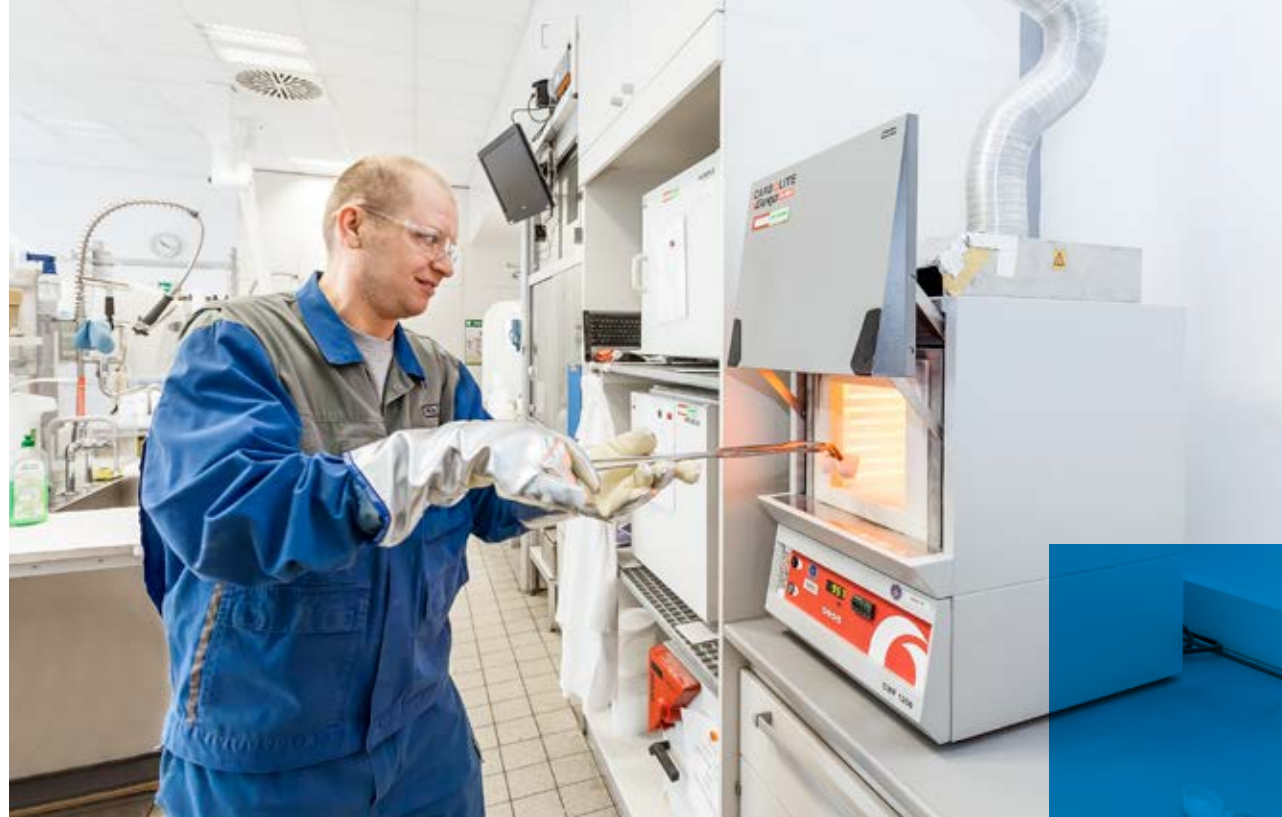
Thomas Seitz at the muffle furnace for determining ash content: since the furnace reaches temperatures of up to 1,000 degrees Celsius, the lab assistant must cover his entire body and wear extra-long, heat-resistant protective gloves.
