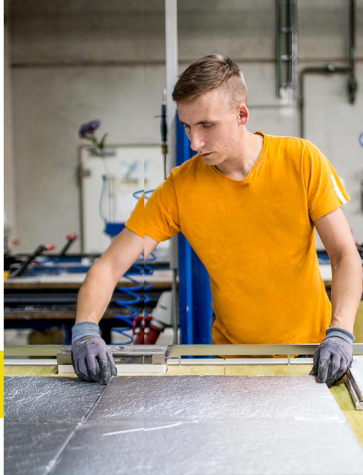
Finished vacuum insulation panels at Ilseburg-based Vitec in Germany, waiting to be packed. Creating a vacuum increases the insulating effect of the processed insulation material by roughly a factor of seven.
