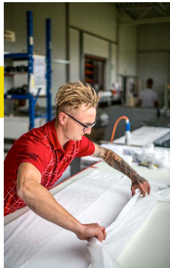
An employee prepares an insulation panel so that it can be packed in protective film and then have a vacuum applied to it.
