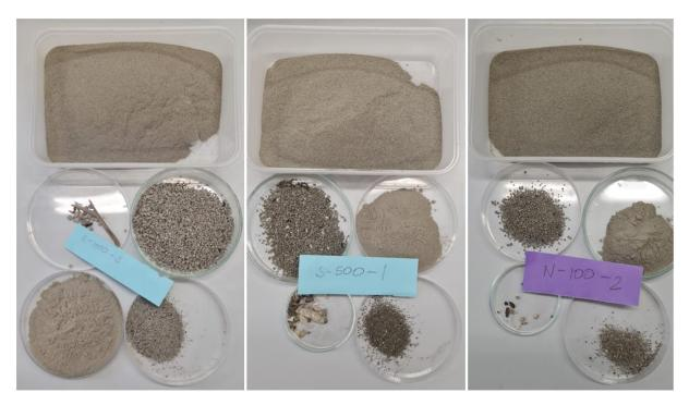
Figure 3-4: Photograph of examples of the five Wentworth sediment composition classification levels at three sampling stations.
