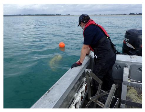
Figure 3-2: Deploying the drifting drogue for water quality sample collection.
