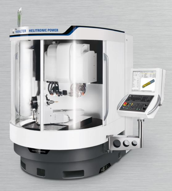
HELITRONIC POWER – the space-saving version with a belt-driven spindle and two ends. The most economical solution for many production and regrinding companies.
