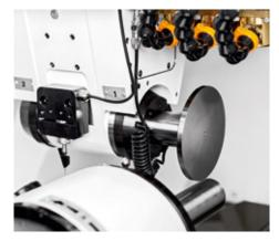
**Automatic grinding wheel measurement**
