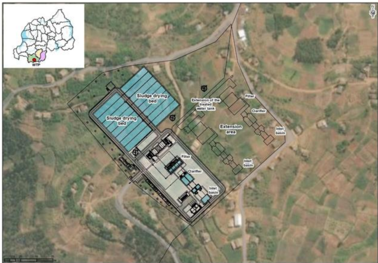
Figure 5: Layout of the proposed WTP
