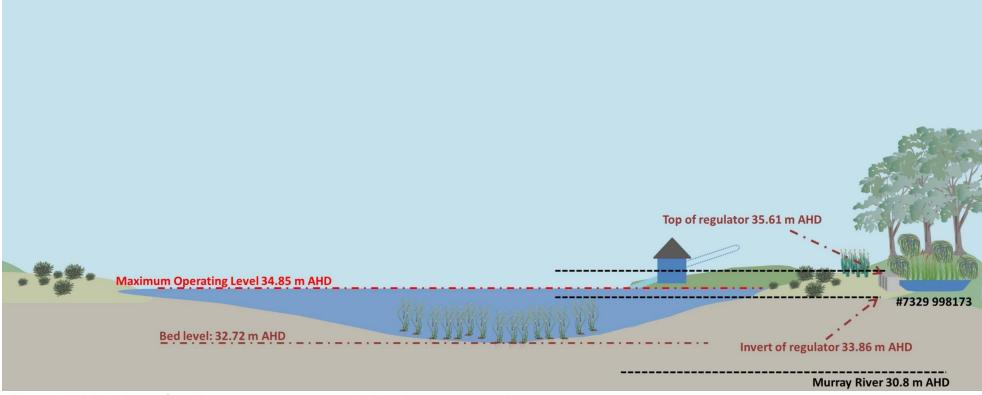
Figure 13. Height datum for relevant components at Lake Hawthorn (not to scale)
