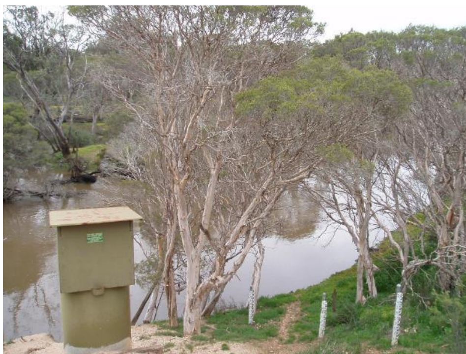
Streamflow gauging station on the Wimmera River at Wail (upstream Dimboola)
