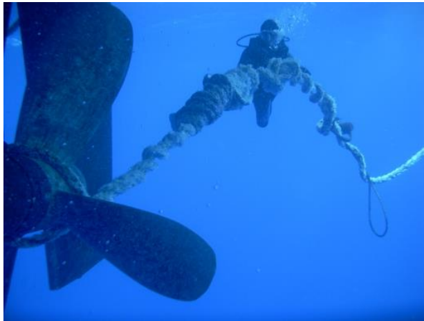
Figure 30. Entangled Propeller (NOAA Marine Debris Program).
