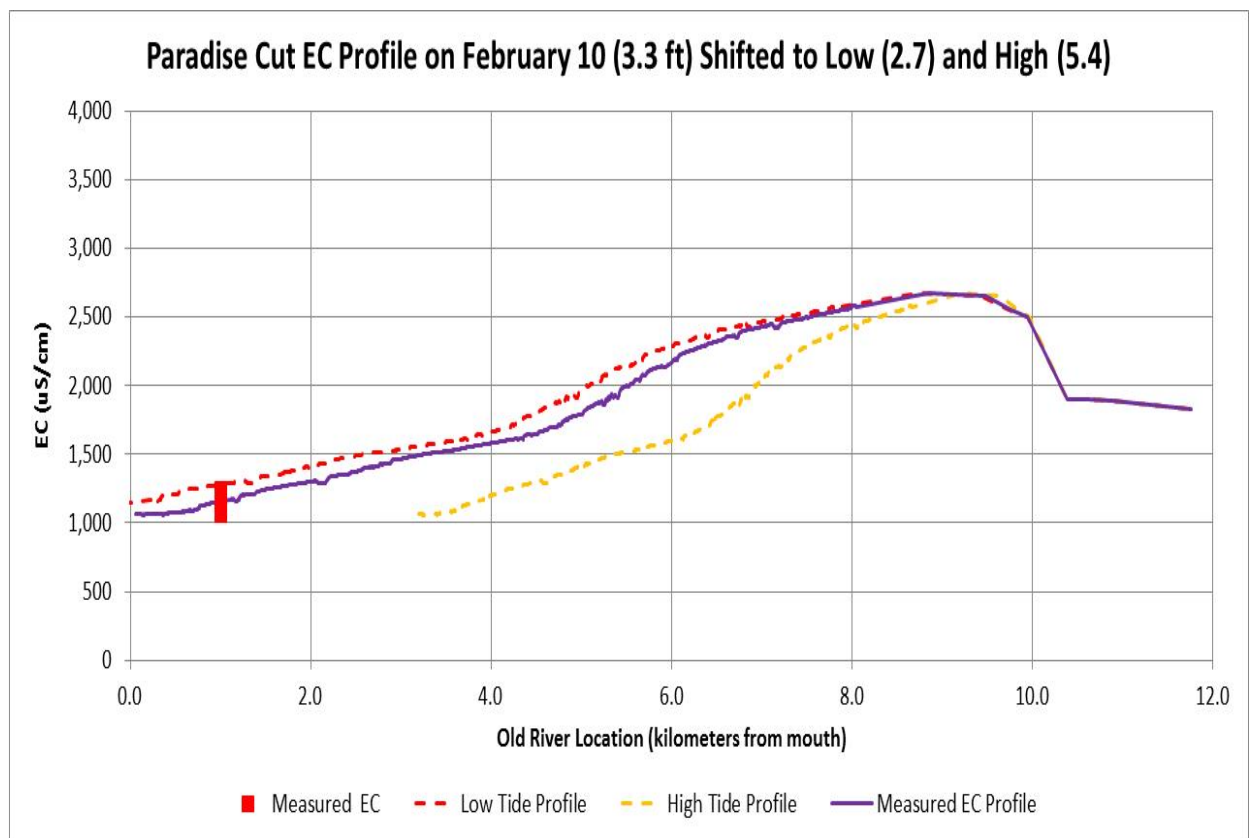
Figure 31a. Measured and Shifted (low and high tide) Paradise Cut EC Profiles on February 10, 2009
