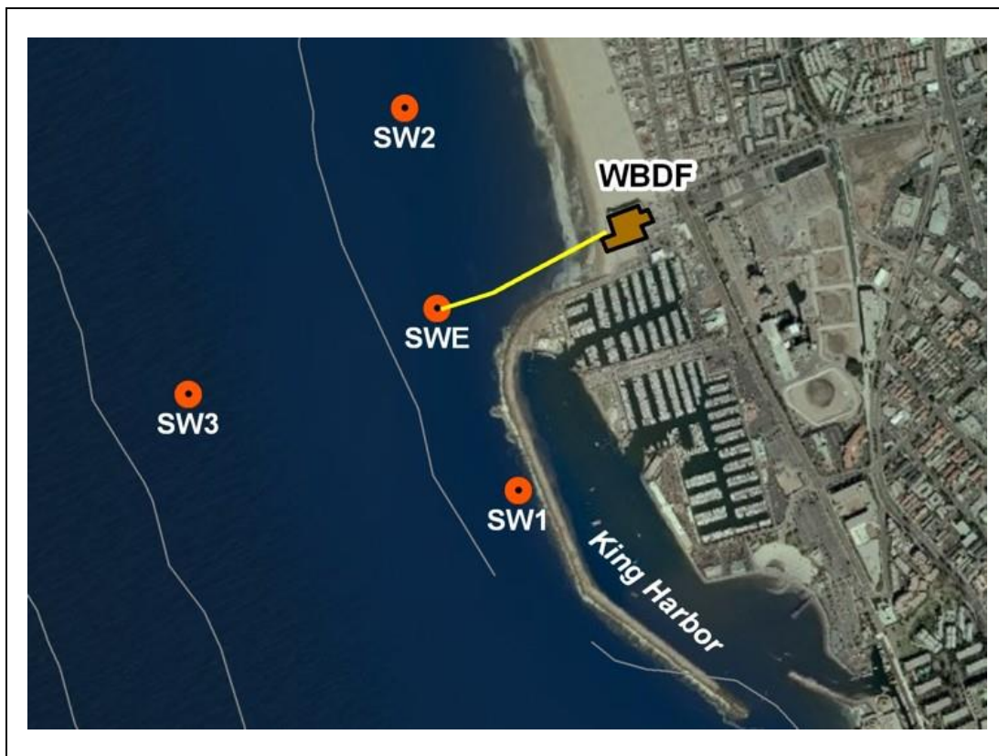
Figure 3-1. Location of intake and source water stations for plankton sampling. Depth contours are at 10 m (33 ft) MLLW intervals.
