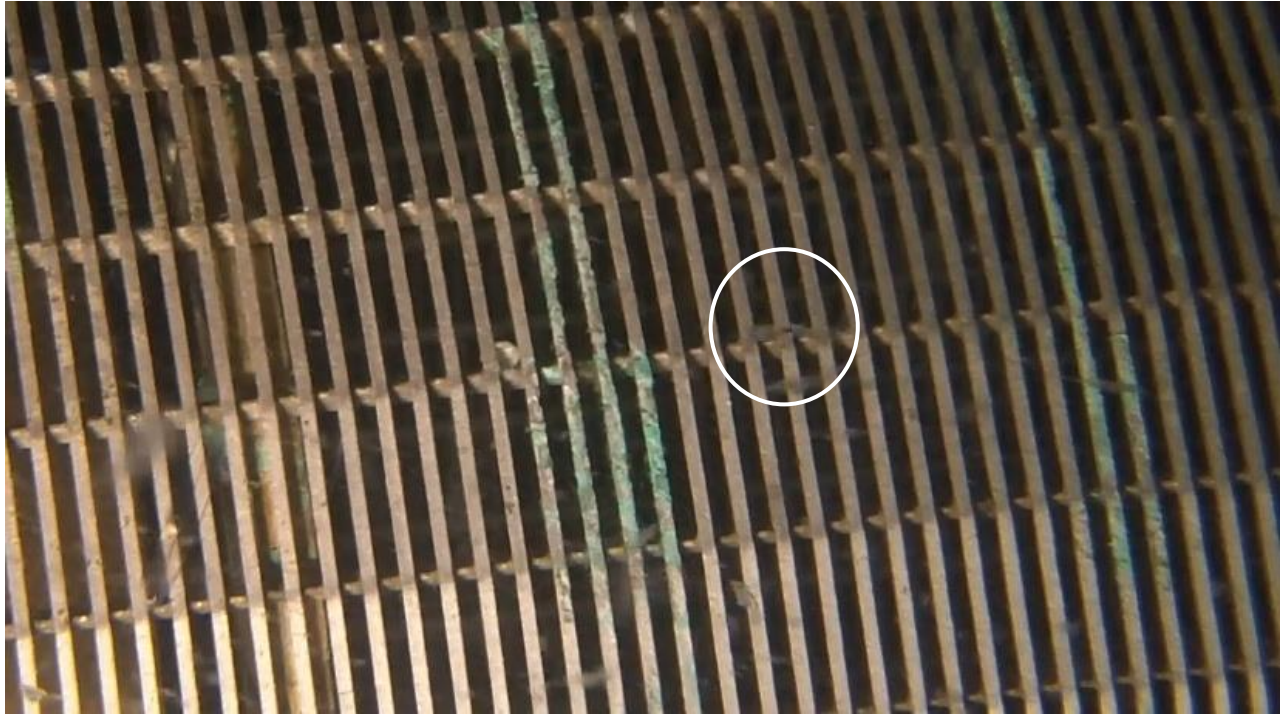
Figure 4-6e. Video frame grab of the 2 mm screen taken in January 2012 during the wedgewire screen efficiency study with the pump operating. Frame shows the fish possibly contacting the screen.
