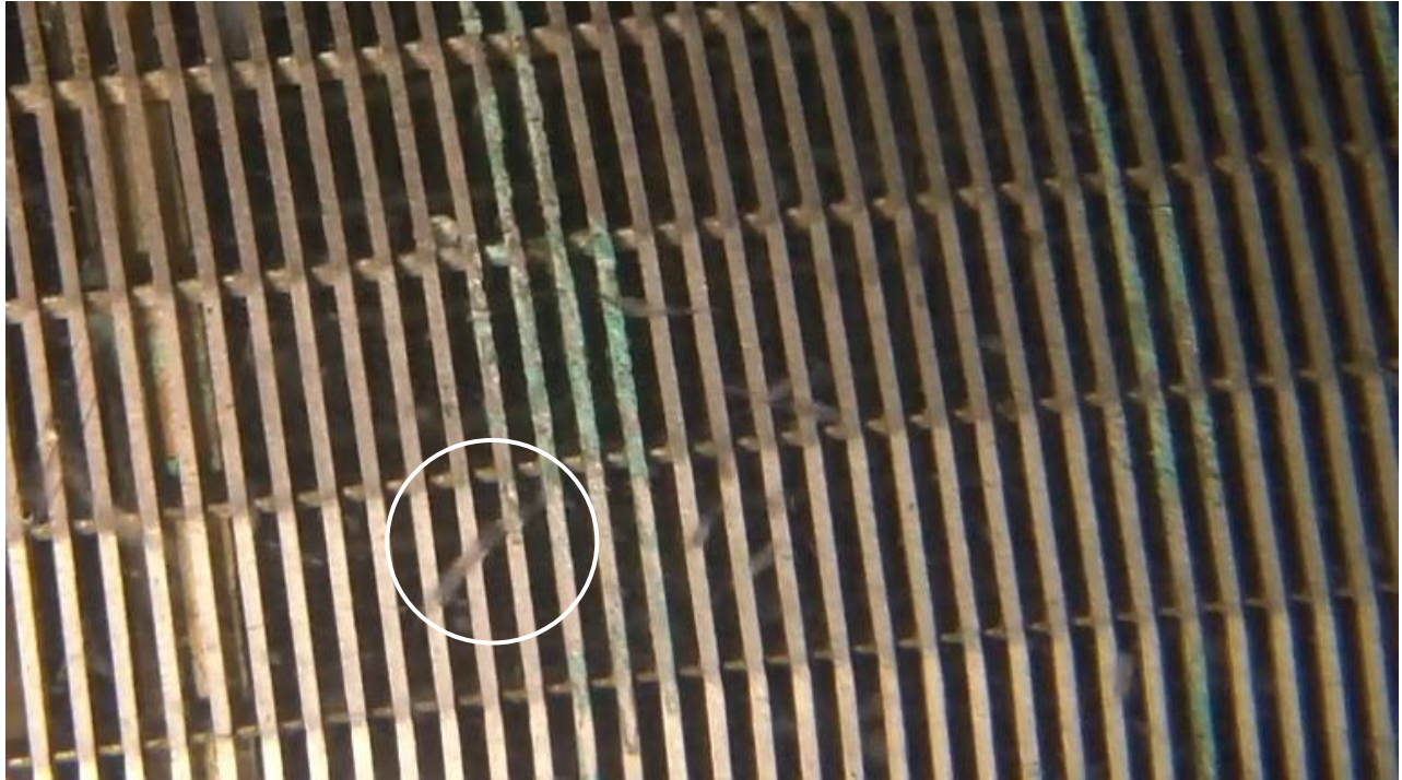
Figure 4-6g. Video frame grab of the 2 mm screen taken in January 2012 during the wedgewire screen efficiency study with pump operating. Frame shows the fish as it moves rapidly away from the screen.
