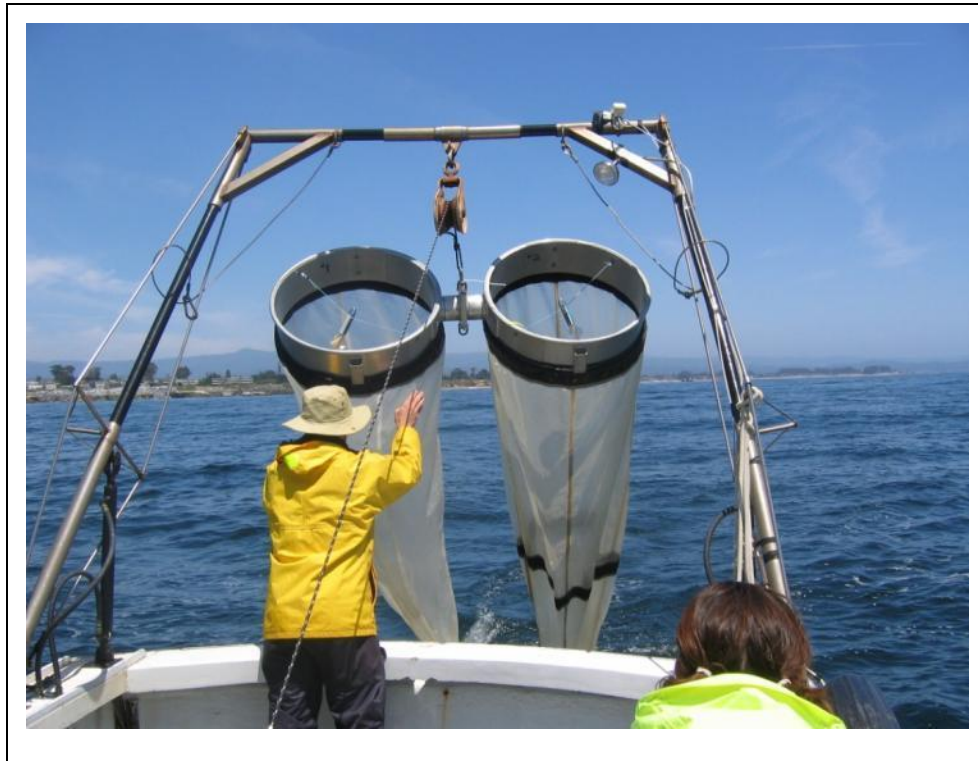
Figure 3-2. Bongo frame and plankton nets used to collect fish and shellfish larvae at the intake and in the source water.
