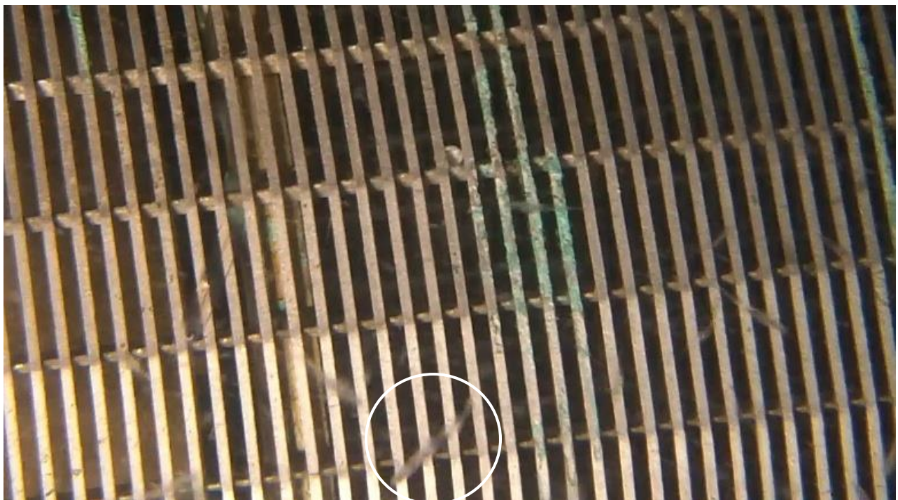
Figure 4-6h. Video frame grab of the 2 mm screen taken in January 2012 during the wedgewire screen efficiency study with the pump operating. Frame shows the fish as it swims away from the screen and the frequency of its tail beats slows.
